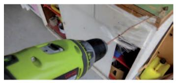
With a nail or screw fastened to a sturdy work bench, place the loop of the wire over the nail/screw and firmly clamp the other end of the wires into an electric drill or old hand drill.
