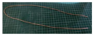
Here I am using a piece of copper wire, approx 2mm thick. You could use pretty well any kind of wire as long as it is easily bent and twisted.
