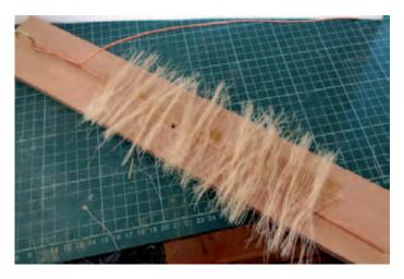
Using a piece of scrap timber, twist a CUP HOOK into the top of the board to hold your copper wire — make a loop twist in the wire and slip it over the cup hook. Lay out the wire as shown above and the place a bead of strong glue, such as Liquid Nails or similar construction adhesive, onto the bottom most wire.
